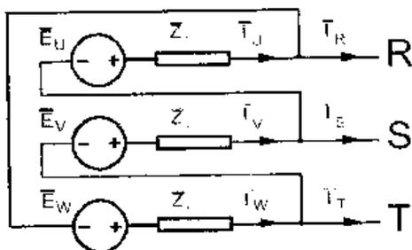
Sol: (a)  $I_U = 10 \angle 30^\circ$  A ;  $I_V = 10 \angle -90^\circ$  A ;  $I_W = 10 \angle 150^\circ$  A, (b)  $U_R = 127 \angle 90^\circ$  V ;  $U_S = 127 \angle -30^\circ$  V ;  $U_T = 127 \angle -150^\circ$  V ; c)  $Z_Y = 0 + j 7.33 \Omega$
