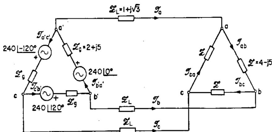
Sol: I de FASE:  $I_{ab} = \frac{40}{\sqrt{3}} \angle -30^\circ$  ;  $I_{bc} = \frac{40}{\sqrt{3}} \angle 90^\circ$  ;  $I_{ca} = \frac{40}{\sqrt{3}} \angle -150^\circ$  A ( $I_{b'a'} = I_{ab}$ ;  $I_{c'b'} = I_{bc}$ ;  $I_{a'c'} = I_{ca}$ ).
