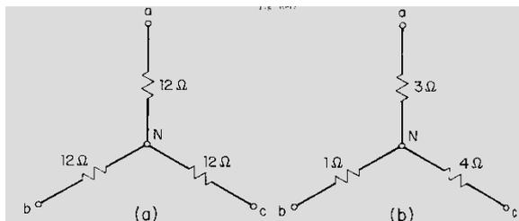
Sol: (a)  $Z_{\Delta}= 36 \Omega$  ; (b)  $Z_{ab}= 19/4 \Omega$  ;  $Z_{bc}= 19/3 \Omega$  ;  $Z_{ac}= 19 \Omega$
