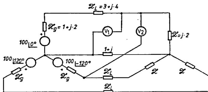
Sol:(a)  $|V1| = 22.36$  V ( $V1 = 10\sqrt{5} \angle 26.6^\circ$  V) ;  $|V2| = 94.5$  V ( $V1 = 94.5 \angle 52.5^\circ$  V), (b) P (carga) = 0 W, (c) R = 750 VAR
