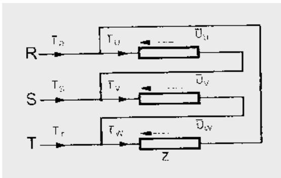
Sol: (a)  $U_U = 381 \angle 120^\circ$  V ;  $U_V = 381 \angle 0^\circ$  V ;  $U_W = 381 \angle -120^\circ$ , V (b)  $I_R = 8.66 \angle 30^\circ$  A;  $I_U = 5 \angle 60^\circ$  A, (d)  $S_U = 1905 \angle 60^\circ$  VA = (952.5 + j1649.8) VA
