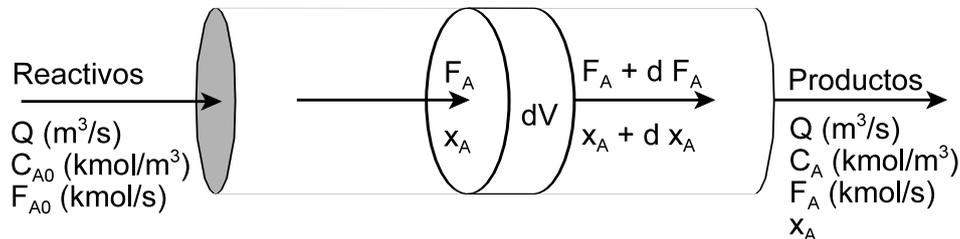
**Figura 5.4:** Reactor tubular.
