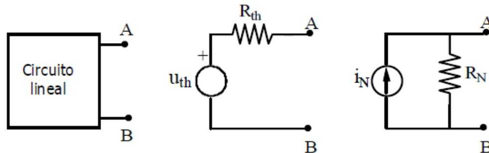
$$R_N = R_{th} \quad i_N = \frac{u_{th}}{R_{th}}$$
