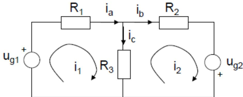
$$\left. \begin{aligned} -u_{g1} + i_1 R_1 + (i_1 - i_2) R_3 &= 0 \\ -u_{g2} + i_2 R_2 + (i_2 - i_1) R_3 &= 0 \end{aligned} \right\}$$
