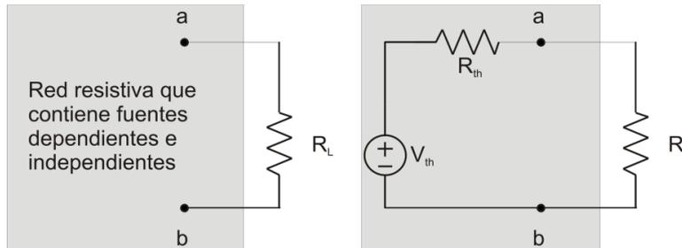
$$p = i^2 R_L = \left( \frac{V_{th}}{R_{th} + R_L} \right)^2 R_L$$
