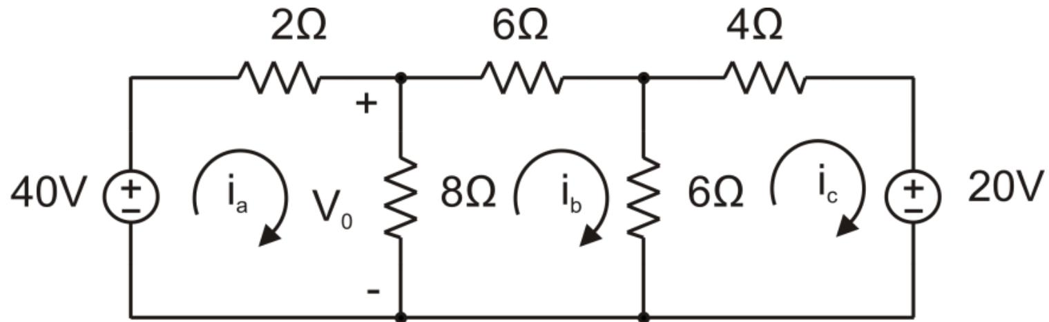
$$\left. \begin{aligned} 40 &= 2i_a + 8(i_a - i_b) \\ 0 &= 6i_b + 6(i_b - i_c) + 8(i_b - i_a) \\ -20 &= 4i_c + 6(i_c - i_b) \end{aligned} \right\}$$
