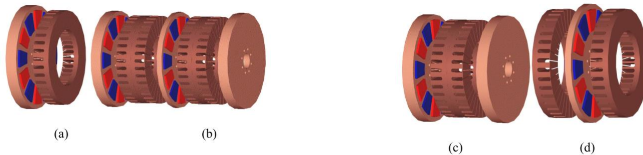
Fig 1 Different structures for AFPM machines, a) Structure with one rotor and one stator, b) Multi-disc structure, c) TORUS type, and d) AFIPM type.
