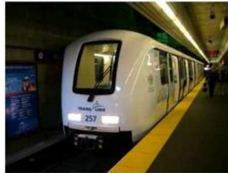
(b) Subway driven by linear motors.
