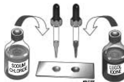
Fig. 4.3 Adding a drop of saline and a drop of iodine suspension to the slide
