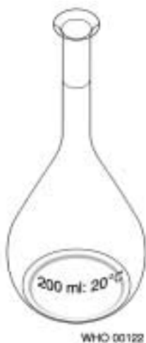
Fig. 3.53 Mark the temperature at which the reagent should be measured on the flask
